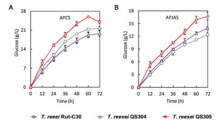
Fig. 6. Hydrolysis of APCS (A) and APJAS (B) by cellulases produced by *T. reesei* QS305, QS304 and Rut-C30. Data are represented as the mean of the triplicate with standard deviations.
